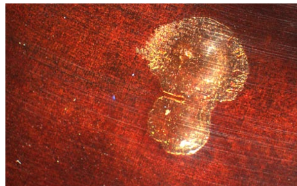
Figure 7. Sampled blister retained distorted conformation after removal of PEG. Plastic deformation of the epoxy film was confirmed.
