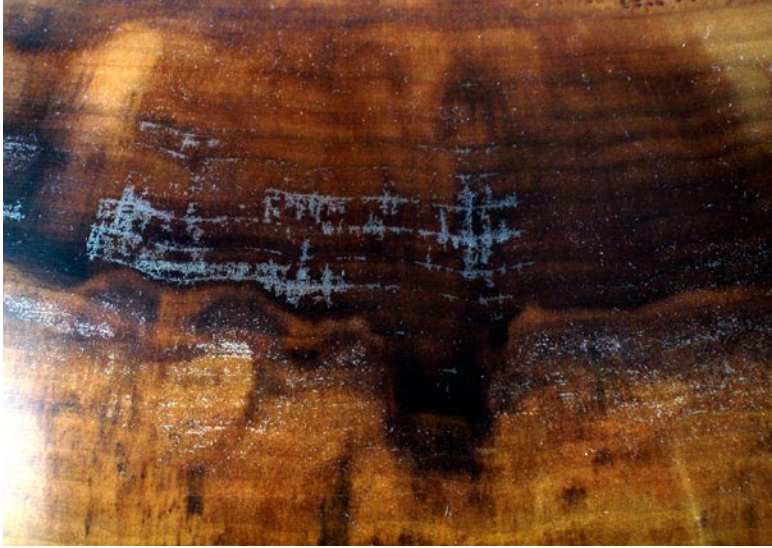
Figure 6. Fractured finish was primarily related to growth rings.
