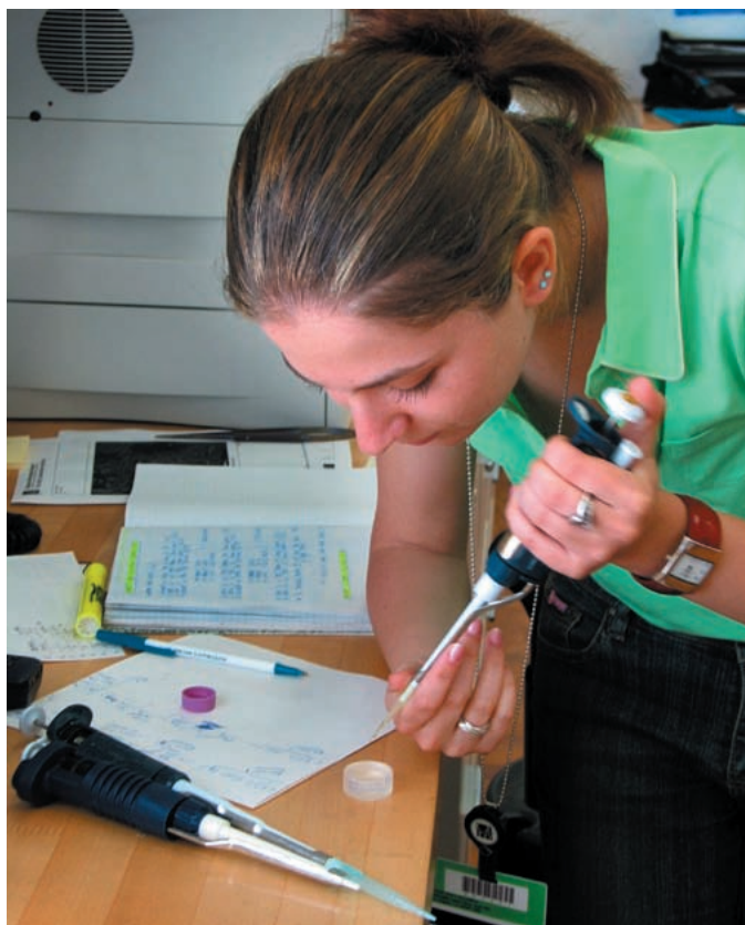
Figure 8. Applying antibodies to a polished cross-section by pipettor.
