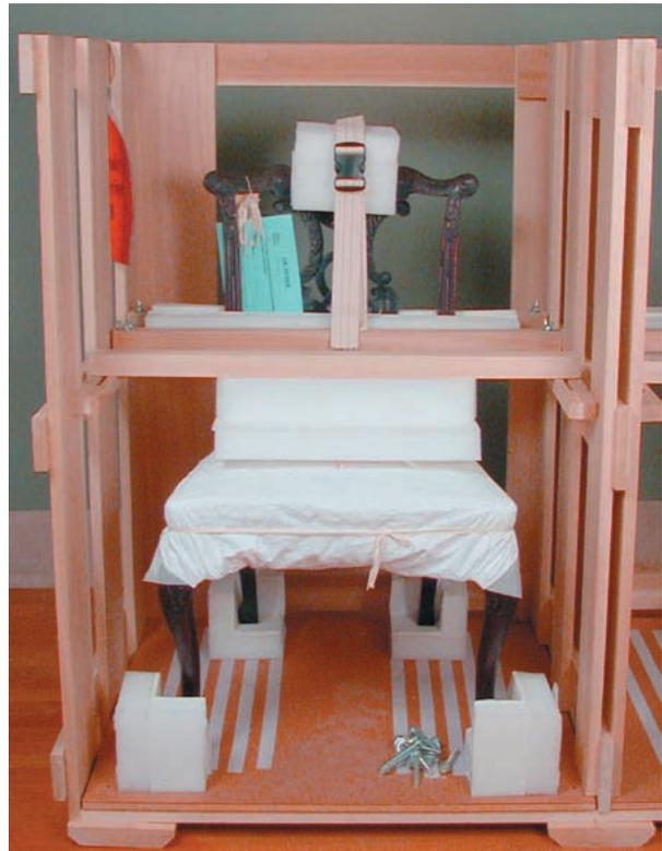
*Figure 8. Additional batten and foam cushion resting on seat.*
