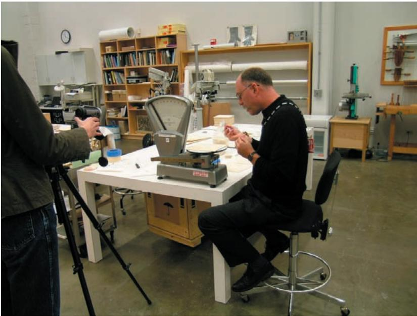
*Figure 6. Digital video camera records the measurement of force exerted on the stage of the analog scale in 30-second sessions.*
