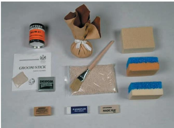
*Figure 3. (left) Cleaning materials: (clockwise from the top right hand corner) Chemical sponge, hard and soft Wishab sponges, three eraser blocks: (Magic Rub, Staedtler Mars and Art Gum), Kneaded eraser, Groom Stick molecular trap, Skum-X, and in the center, grated Magic Rub eraser crumbs.*
