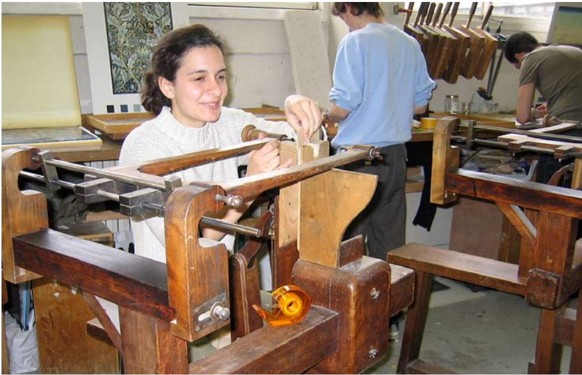
Figure 1. A student at École Boulle operating a marquetry bench. The jaws of the vise have been modified to reduce kerf gap.
