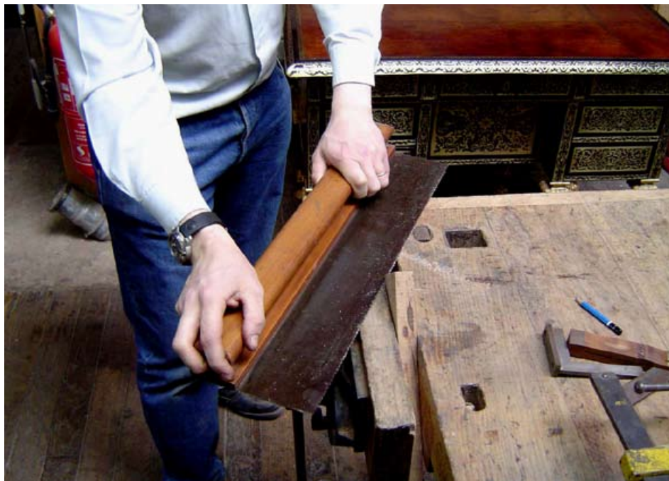
Figure 1. The virtue of this saw is that it can be easily registered against a very broad guiding surface, assuring a very clean and accurate cut. Any laid-out line, angled cut, or even compound angles can be located at the bench or jig top and sawed without any fussy setup or gauging. A fixture such as a shooting board would be the best way to use this saw, but by no means essential if the bench top is flat and square to the vise.
