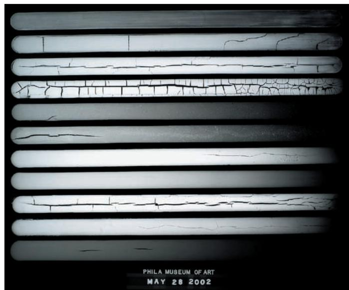
FIG. 2 The eleven test gesso formulations in table 2.
