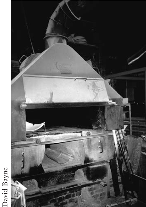
Wood fired 19th-century kiln for slumping glass into forms. Patrick Desserre glass, Paris
