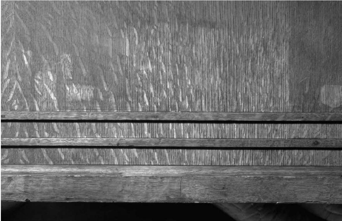
*Figure 7: A cleaned area of the sofa finish that had darkened due to polishing and environment.*
