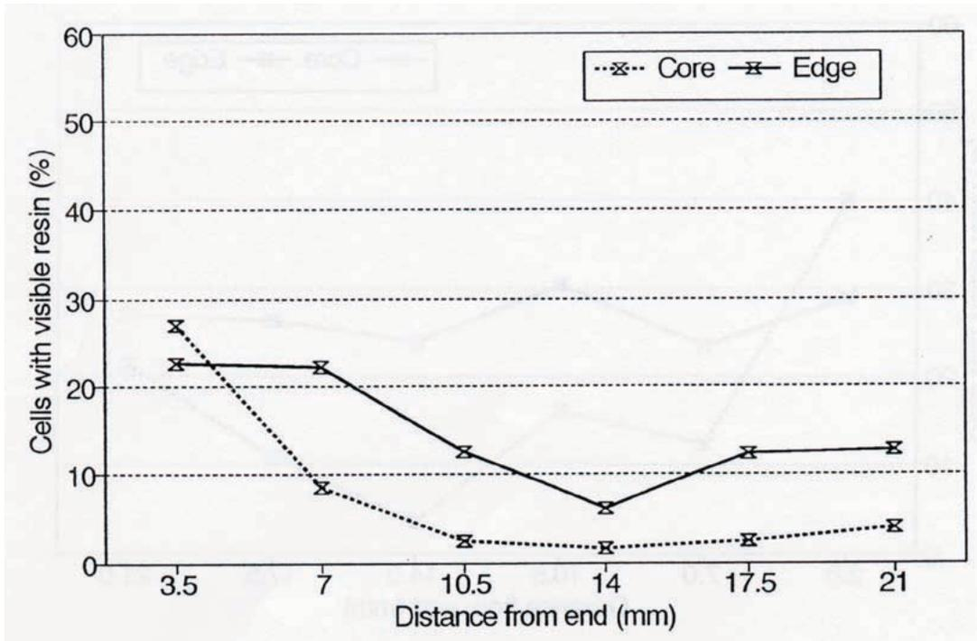
**Figure 6.** Percent of cells with visible resin in specimens treated with 20% B72 in toluene vs. location.
