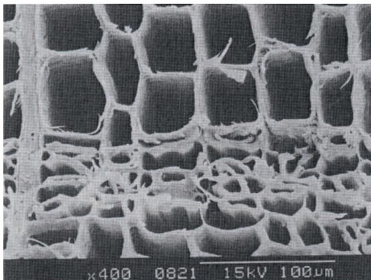
**Figure 2.** Cross section of deteriorated, untreated Douglas-fir showing nearly destroyed latewood below and apparently intact earlywood above. Note spiral thickenings inside the earlywood cells.
