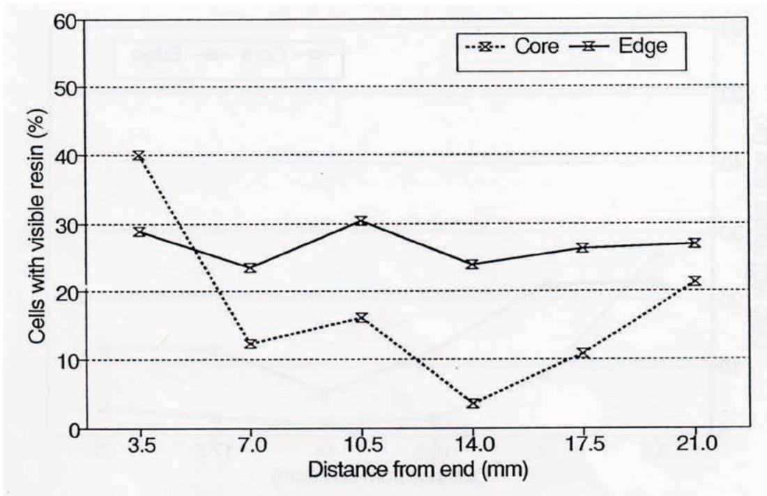
**Figure 8.** Percent of cells with visible resin in specimens treated with 20% B98 in ethanol/toluene vs. location.
