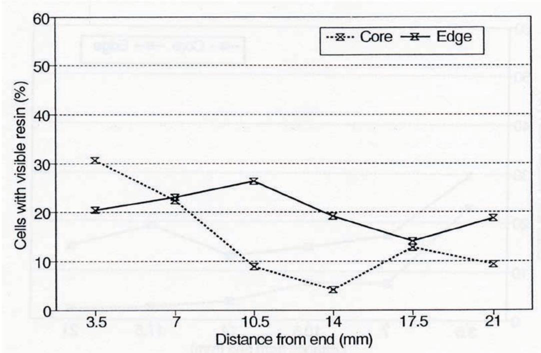
**Figure 7.** Percent of cells with visible resin in specimens treated with 20% B98 in ethanol vs. location.
