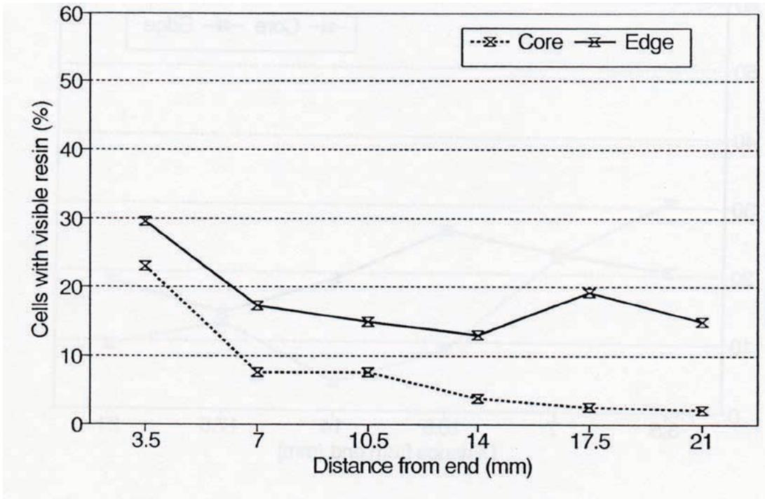
**Figure 5.** Percent of cells with visible resin in specimens treated with 20% B72 in acetone vs. location.
