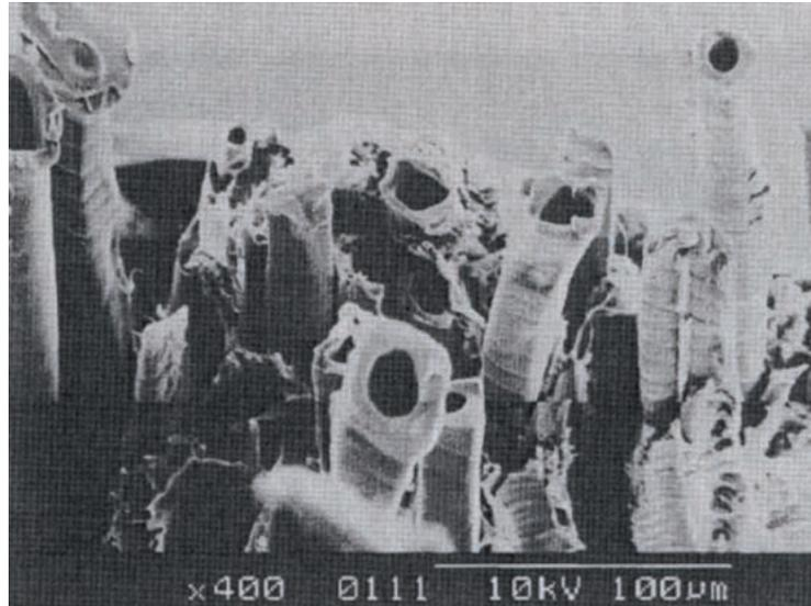
**Fig. 4.** Fracture surface of specimen treated with B98 in ethanol 3.5 mm from the end and close to the edge, showing sleeves and plugs protruding beyond the fracture plane.
