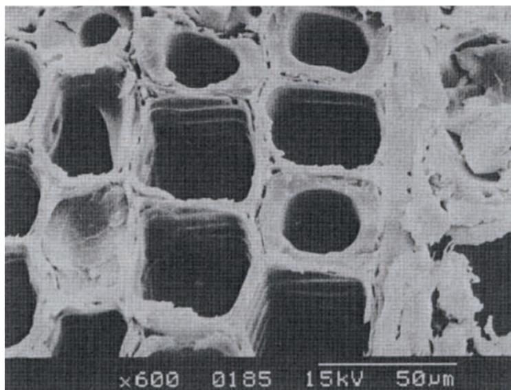
**Figure 3.** Earlywood cells treated with 20% B72 in toluene. Note solid plug in cell at lower left and thick sleeves of resin toward the top. Spiral thickenings clearly visible in other cells indicating little or no resin content.
