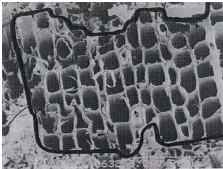
**Figure 1.** Sample area of 73 cells containing 19.2% cells with plugs or sleeves of consolidant (B98 in ethanol).
