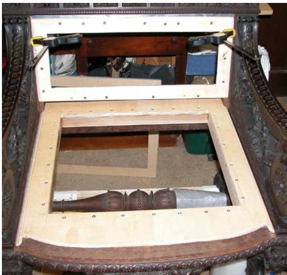
Figure 6. New Baltic birch plywood and sweetgum insert frames.
