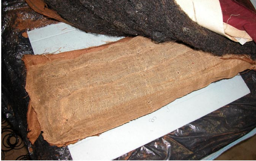
Figure 5. Original under-upholstery materials in the back. horizontal web, foundation jute cloth, and a fixed bridle-stitched back cushion of a coarse white fabric and curled hair. The curled hair stuffing in the seat and back may be original and reused in subsequent reupholstery campaigns. Much of the existing curled hair had been infested with carpet beetles at some point. These materials are no longer actively infested and pose no risk as long as they are bagged and boxed.
