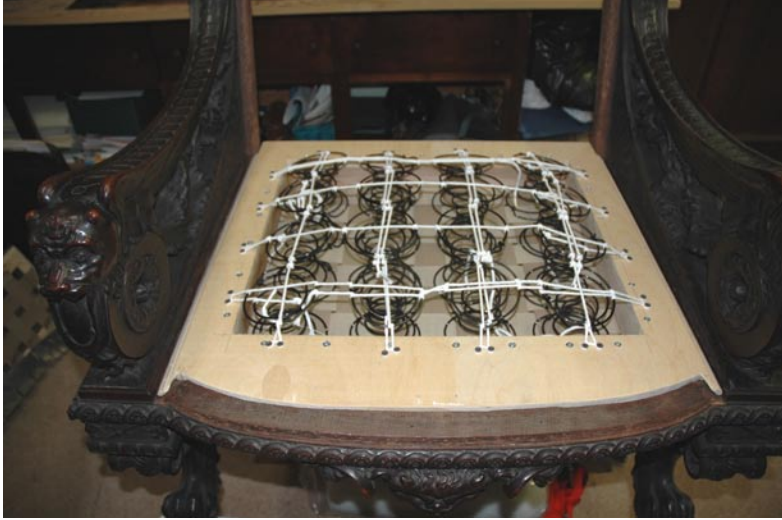
Figure 7. Springs tied to Dacron webbing.
