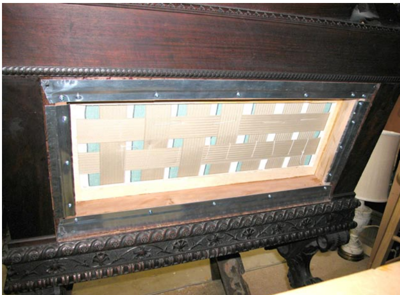
Figure 10. View of outback before the leather cover: back frame with removable aluminum flanges.
