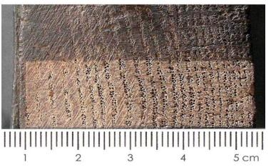
Figure 5. A view of oak end-grain; the lower half has been prepared for measurement by micro-abrasive blasting. Note that the diagonal tool marks are still clearly visible after sample preparation.
