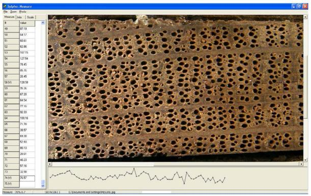
Figure 6. For direct measurement, digitized photomacrographs of prepared end-grain were measured and converted to growth curves using customized Mensor<sup>®</sup> software created in 2002 by S. Meignier and Didier Pousset.
