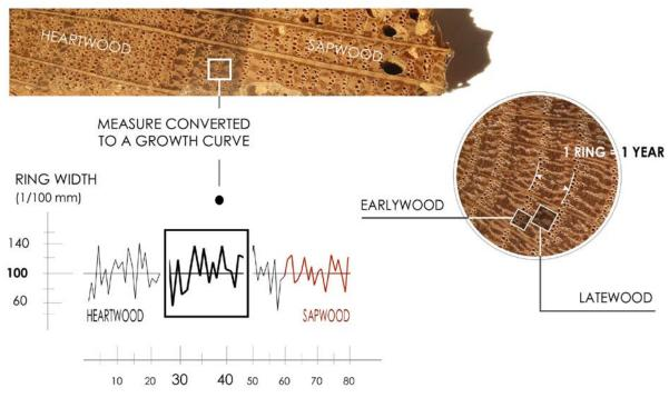
Figure 2. Measurements of individual rings are recorded and used to generate a *growth curve* for each piece of wood studied.
