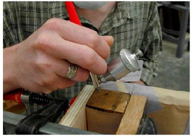
Figure 4. The apparatus for micro-abrasive blasting is similar to an airbrush, offering precise control and portability.
