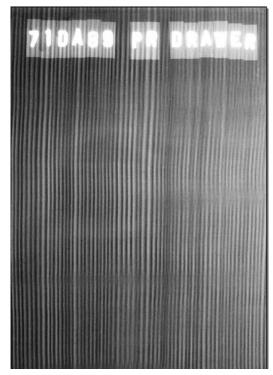
Figure 7. An X-radiograph of a drawer bottom, used to produce a growth curve in a situation where the end-grain of a panel was not accessible.
