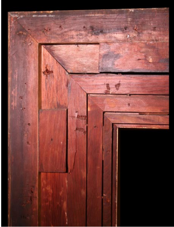
Figure 4. Back view of a four section frame with a box section recess in the main outer profile, and supporting glue blocks.
