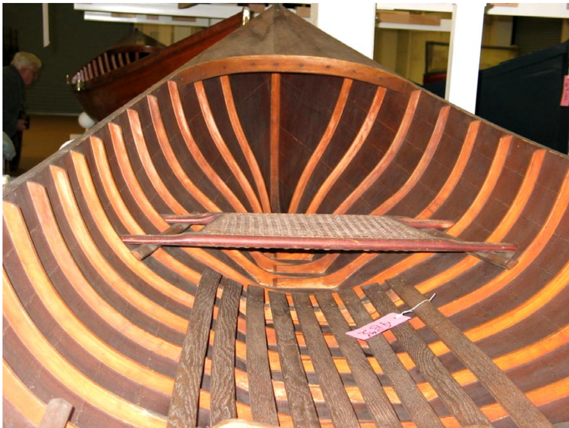
Figure 10. Interior of a guideboat, showing the flat bottom, sawn spruce ribs, and complex curves.
