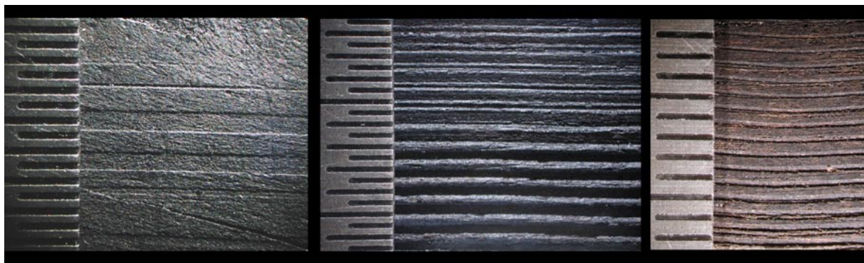
Figure 12. Tothing plane marks found on the ebony cabinet. Original seventeenth-century tothing plane marks (left); first type of nineteenth-century tothing plane marks (center); second type of nineteenth-century tothing plane marks, attributed to Herter Brothers (right).
