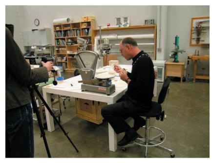
Figure 6. Digital video camera records the measurement of force exerted on the stage of the analog scale in 30-second sessions.
