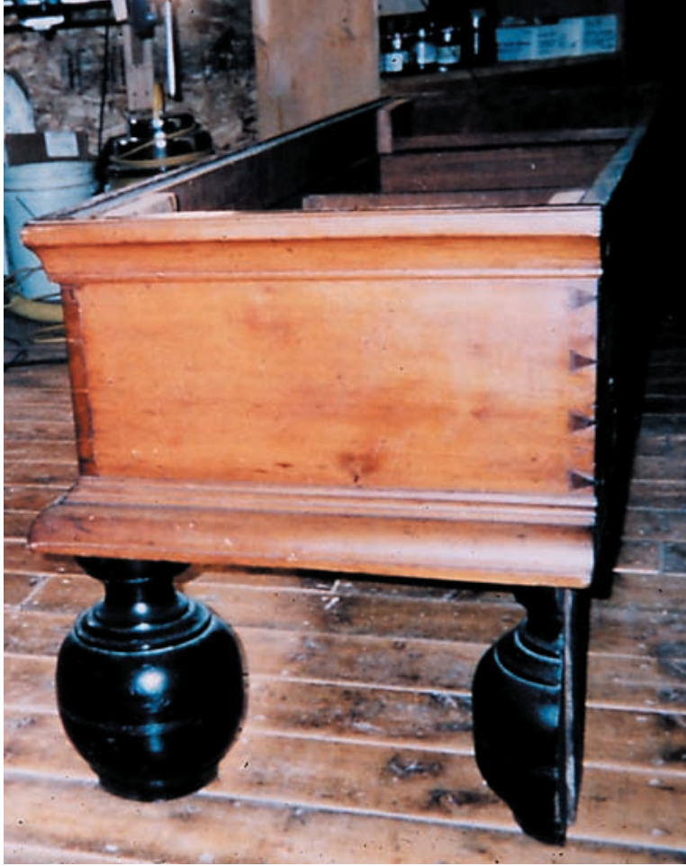
Figure 2. Side of the base section showing the two part dovetailing process. The sides must be joined to the backboard before the front boards can be fit to the sides.
