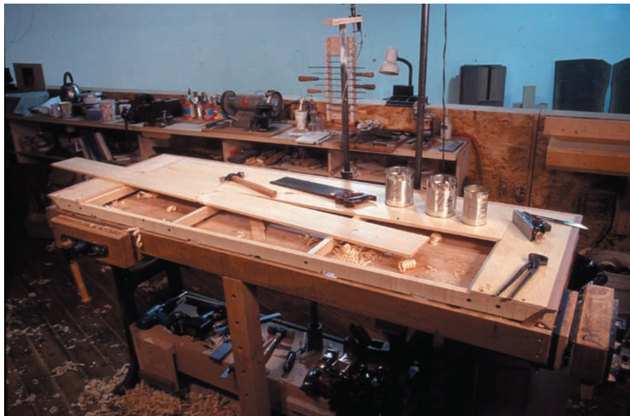
Figure 8. Fitting the top boards to the removable cornice extension.
