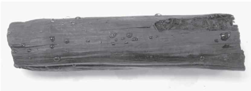
FIG. 4 Example of a waterlogged treenail.
