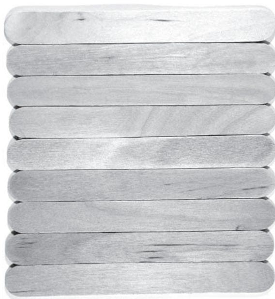
FIG. 6 Control tongue depressor (top); eight MTMS-treated, waterlogged tongue depressors (below).
