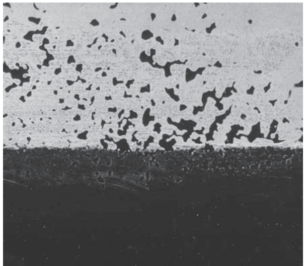
FIG. 4 Detail of the mottled lacquer from the bedroom furniture, showing black laque arrachée filled with a silver-gray lacquer juxtaposed with black lacquer.
