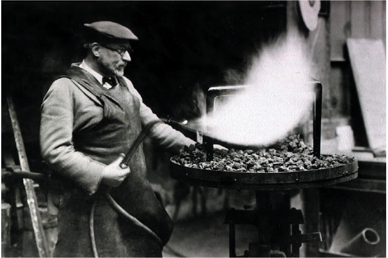
FIG. 11 A 1935 Photograph of Jean Dunand demonstrating with a blow torch the fire resistance of a lacquered table, cast from a gypsum based material containing urushi .
