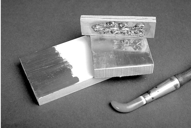
Figure 1. Test blank with Aquazol gesso and bole layers and test blank comparing burnished and unburnished gilded surfaces.
