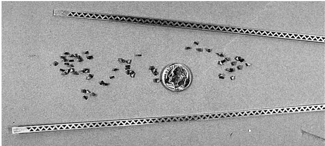
Figure 6. "Zig-Zag" for table in figure 1. The dime gives an idea of the small scale of cut possible with laser milling (this is by no means the limit).
