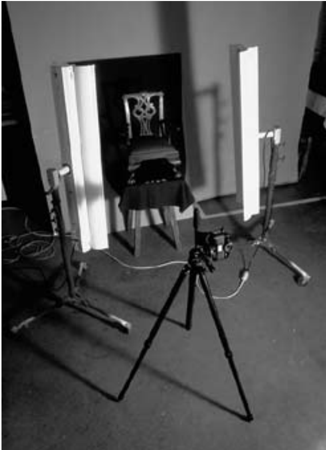
Figure 7 UV induced visible fluorescence photography setup for child's chair with room lights on for illustration.
