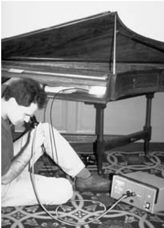
Figure 9 The author using the Olympus Fiberoptic Scope to investigate suspected inscriptions inside the soundbox of a Spinet Harpsichord at Colonial Williamsburg.
