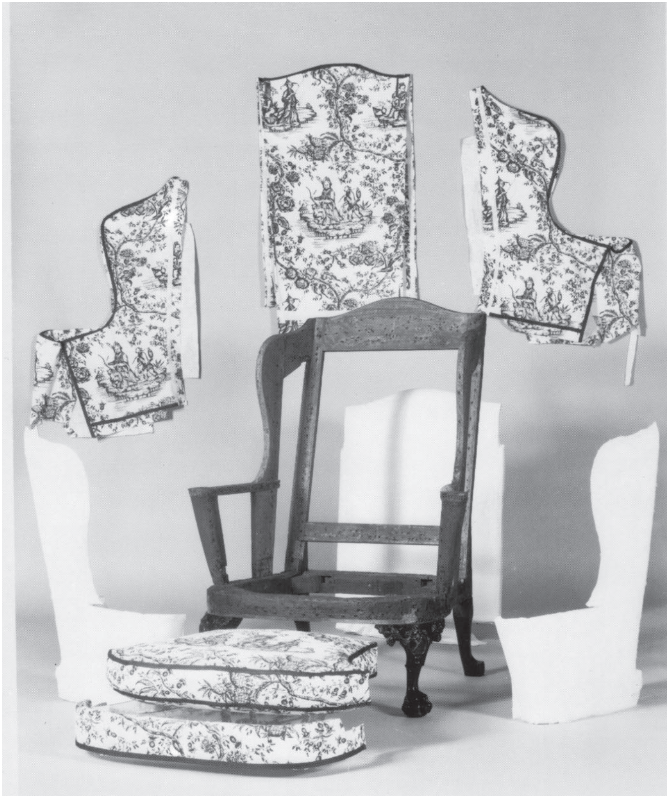
The various components that make up the nail-less, removable upholstery system (three muslin and undercases identical in form to the suspended print cases in the photograph are not shown. There is also a set of show cases made in gold silk. (Photograph courtesy of the Henry Francis du Pont Winterthur Museum.)
